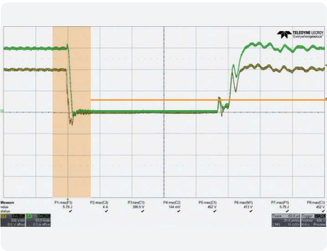
EnerStream 60 generates Arc energy less than 0.2mJ/kW
